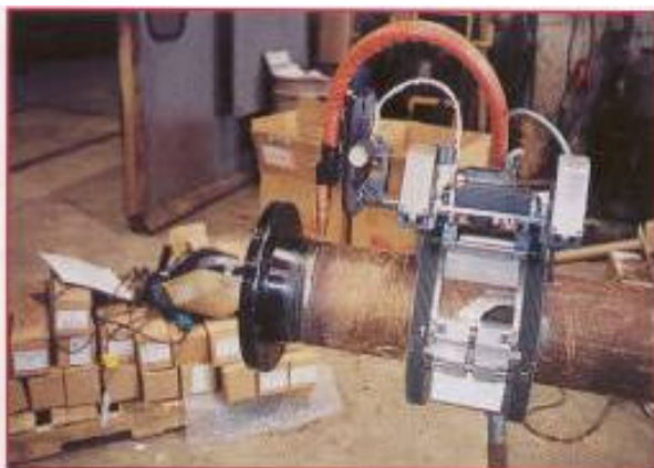
Fig. 1 — Orbital flux cored arc welding machine prepared for use on a pipe section.
